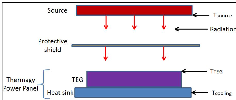
The next specifications are the maximum operating specifications for the complete range of Thermagy™ power panels.
